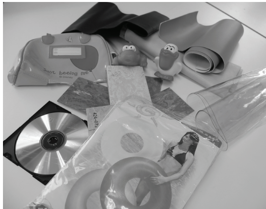
Figure 4. Plastic products (from paper I) which caused toxic leachates, i.e.: artificial leathers (brand S, G and M), children's handbag, bath tub squirt toys, floor material, table cloth (transparent), and inflatable bathing ring. The CD was only toxic when cut into pieces and the silver layer was exposed [I].
