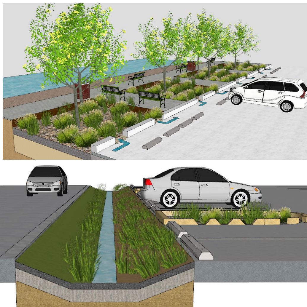
Figure 9: Carpark raingarden and swale examples
