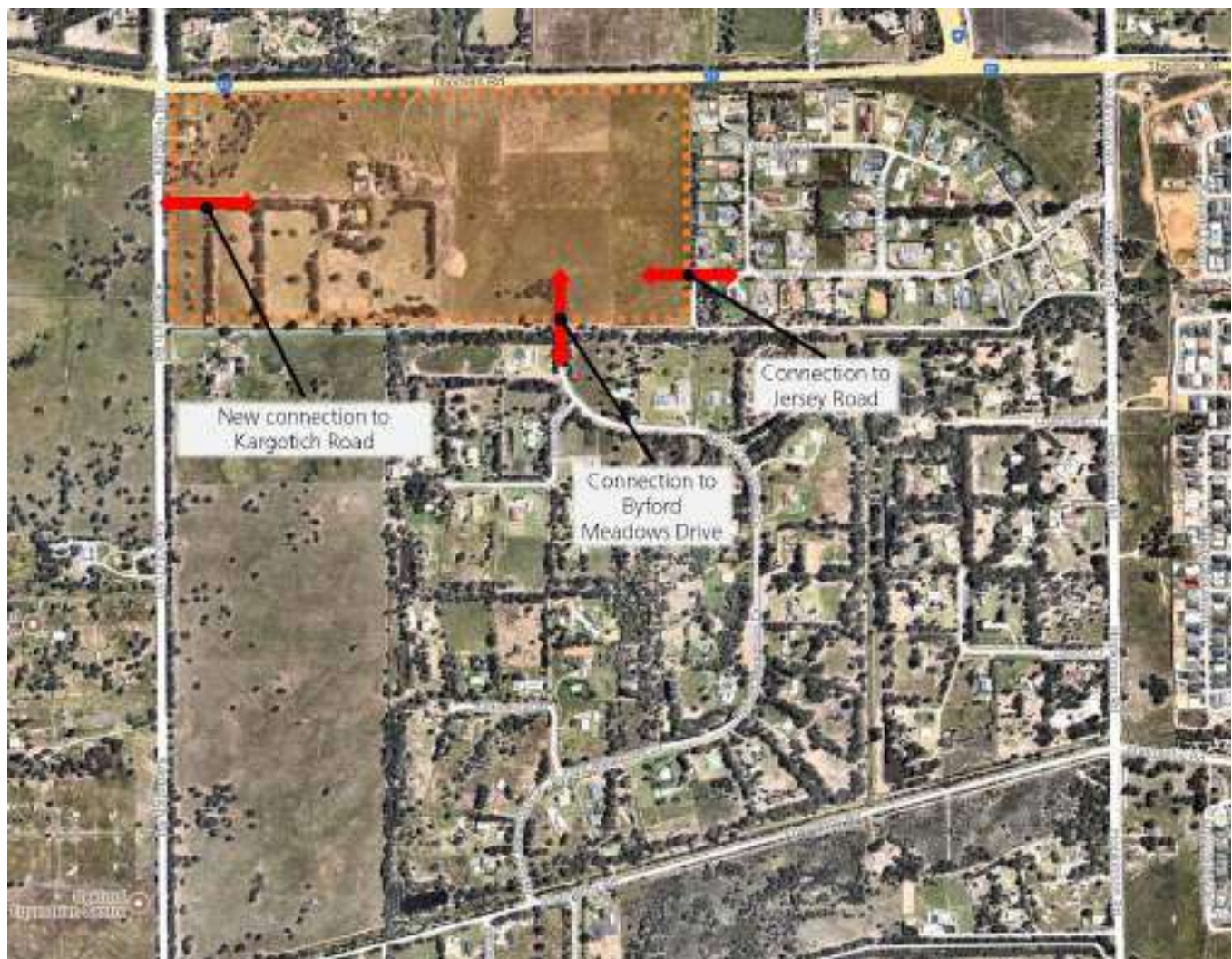
Figure 11 Proposed access arrangements for the subject site shown on aerial image (map source: Nearmap)
