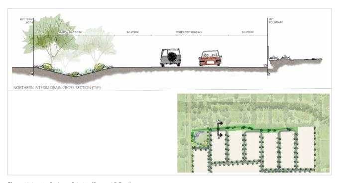
Figure 14: Interim Drainage Solution (Source: LD Total)
