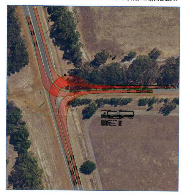
Figure 13: South Western Highway - Kiln Road Intersection Swept Path
