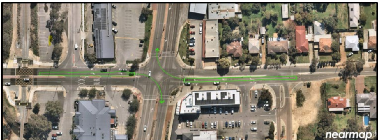
Figure 9: Possible intersection upgrade to Beenyup Road / South Western Highway
