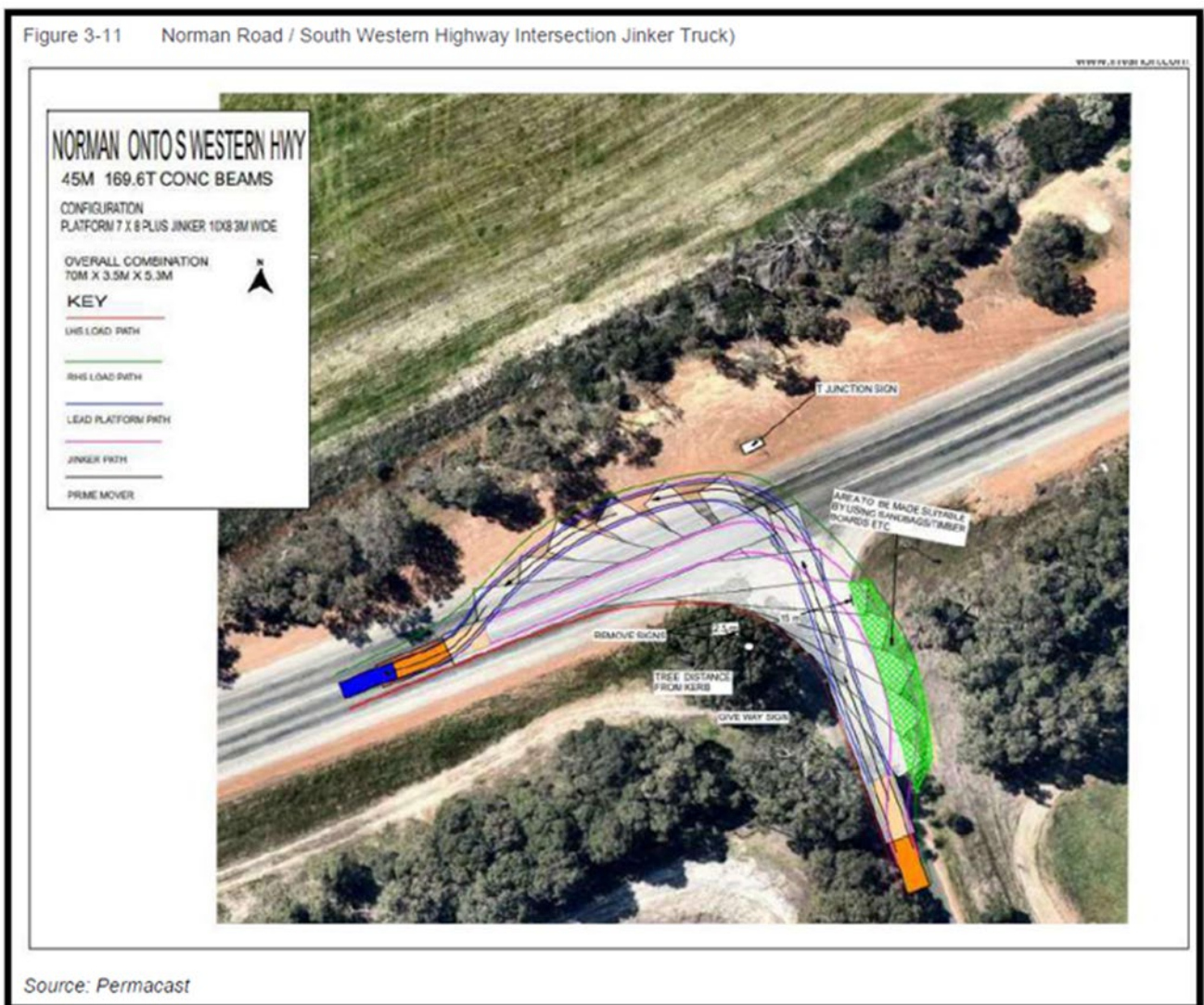
Image 23: 45m Jinker truck swept path diagram - left turn from Norman Road onto South Western Highway
