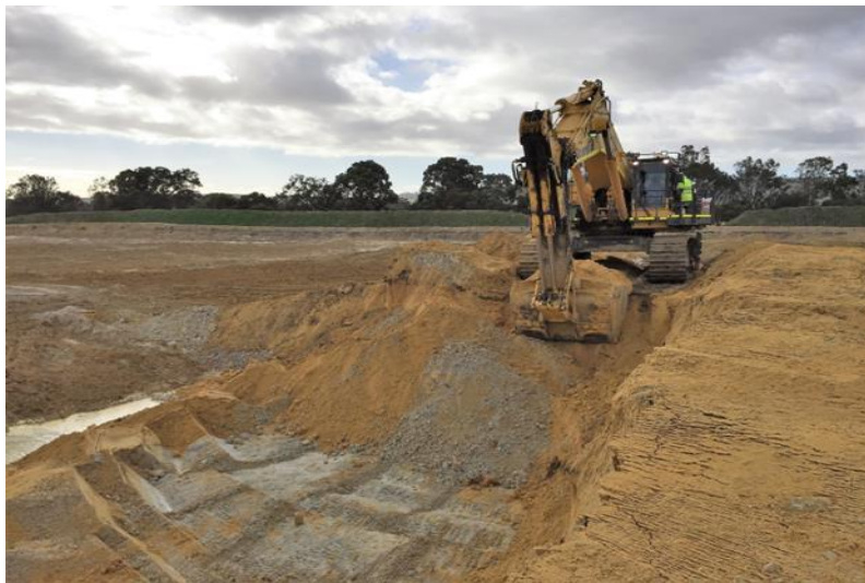
Plate 3: Ore extraction using excavator (note shallow depth of ore body)
