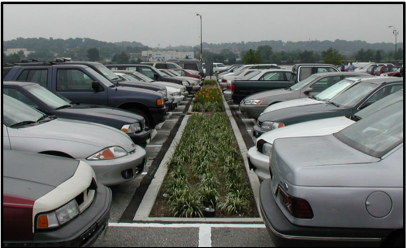
Figure 13: Example of vegetated swale treatment in car parking areas
