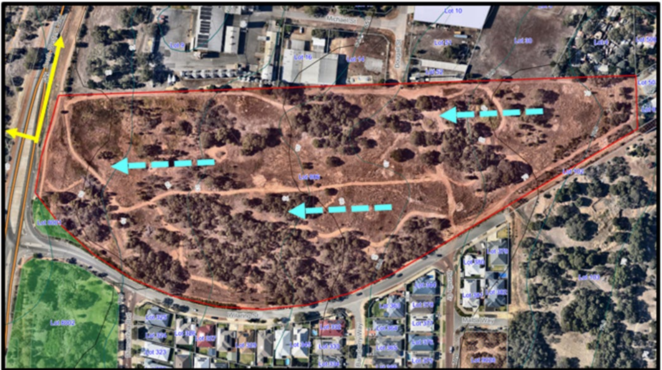
Figure 11: Natural surface/ground water movement (blue) towards the South Western Highway stormwater infrastructure (yellow)
