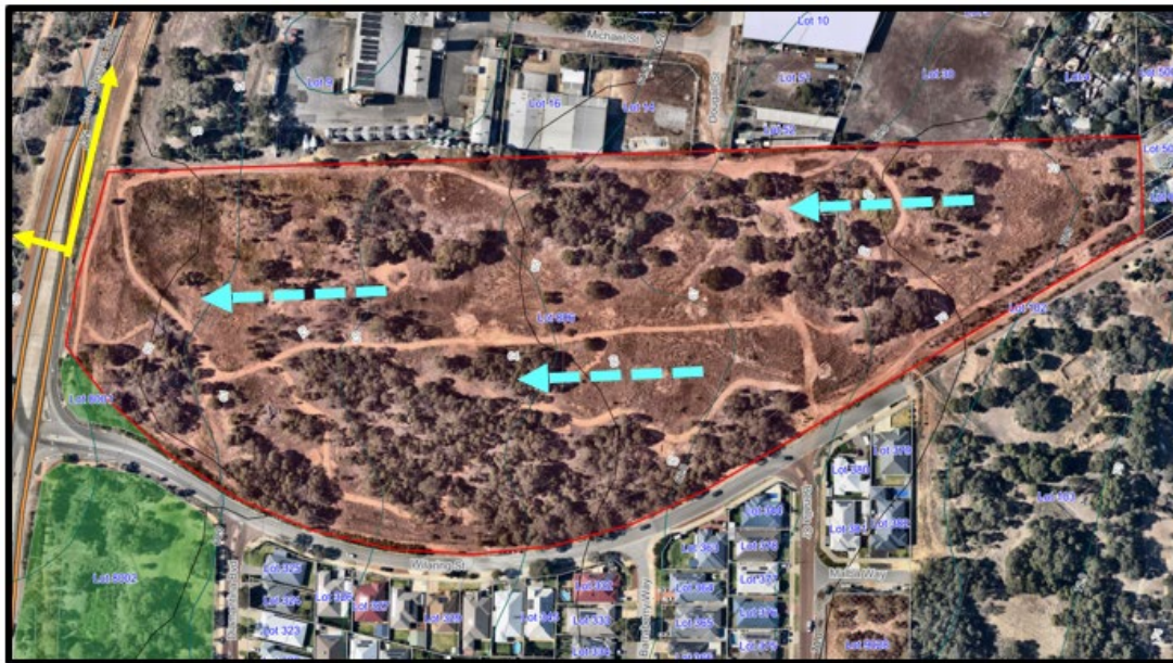
Figure 11: Natural surface/ground water movement (blue) towards the South Western Highway stormwater infrastructure (yellow)
