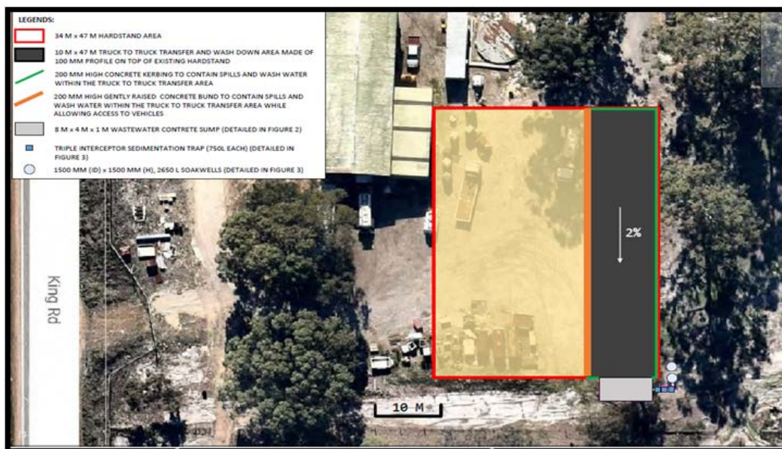
Proposed Raised Kerbed Hardstand Area
