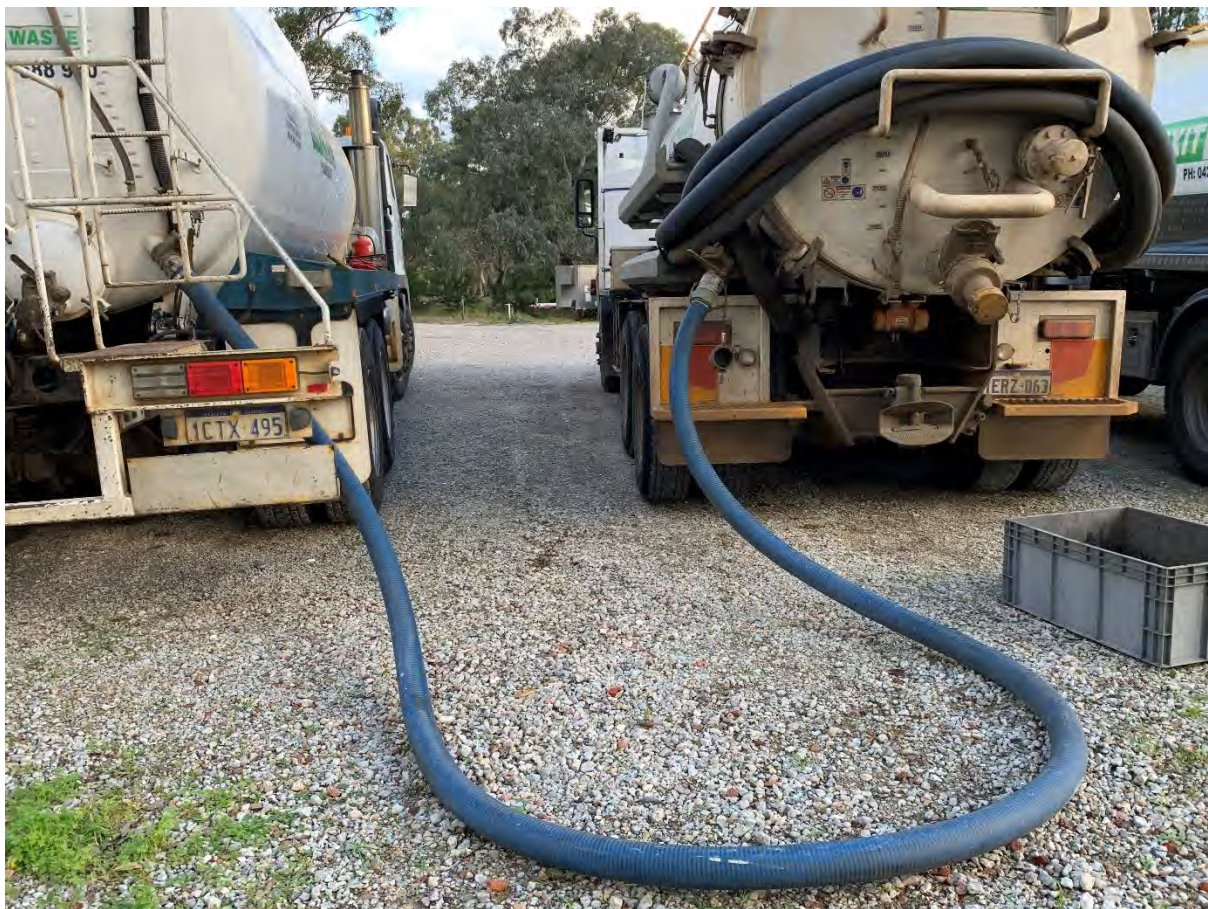
Figure 2.1: Truck to truck decanting via closed coupling
