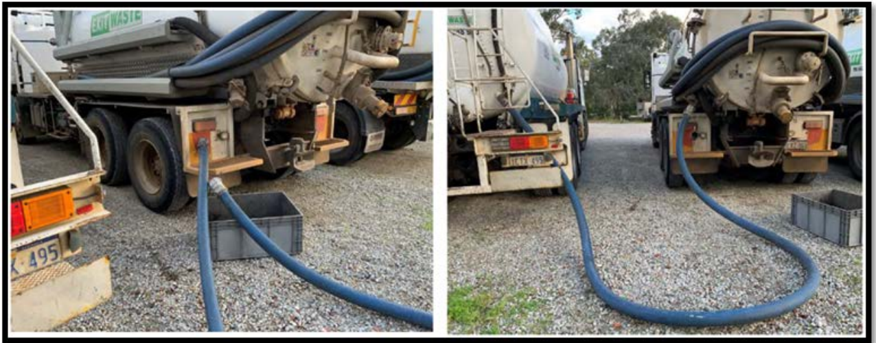
Transfer of Waste from Licensed Controlled Vehicles (Decanting)
