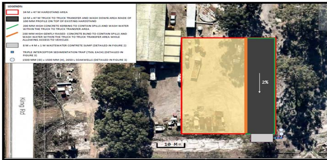
Proposed Raised Kerbed Hardstand Area
