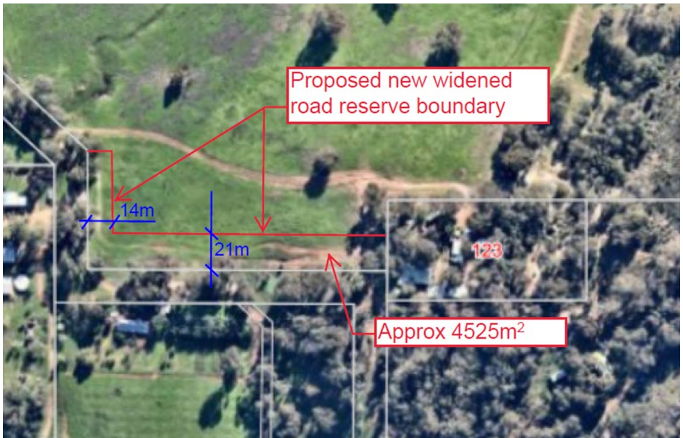
Image C – Portion of Lot 2 to be acquired and amalgamated with Gordon Road road reserve
