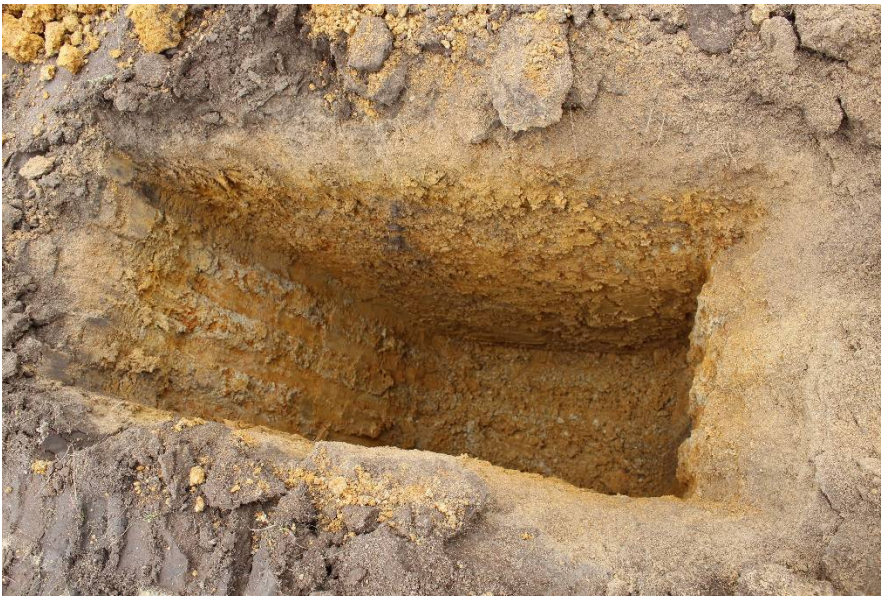
Figure 4.8 (L) Soil profile for test pit 2. (R) Depth to 1500 mm, hard digging.
