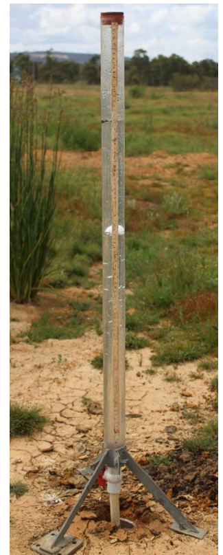
Figure 4.9 (L) Excavated soil. (R) Permeability determination (steady rate).
