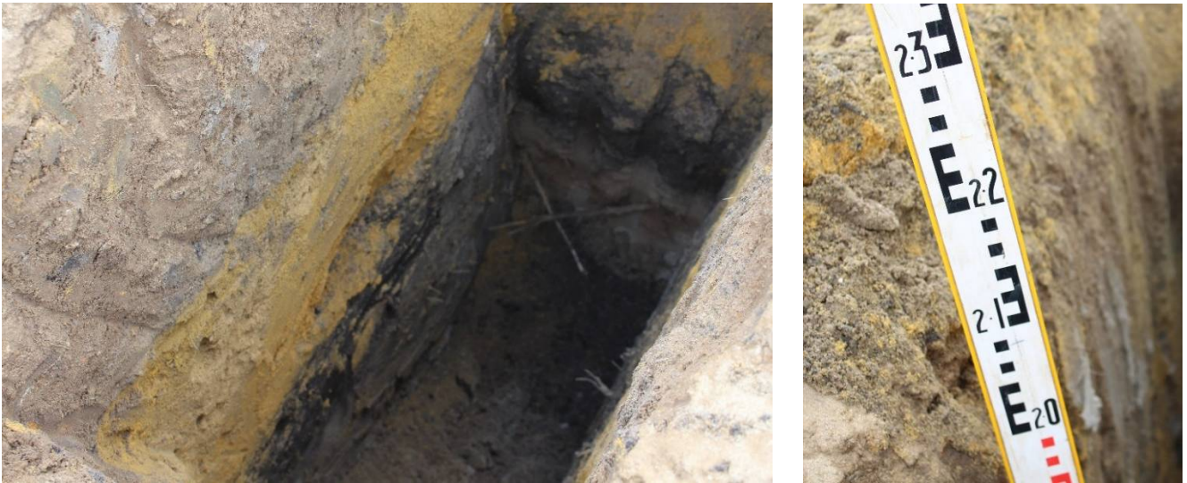
Figure 4.1 Soil profile for test pit 1. Depth achieved 2.2 m before excavation stopped (but no hard digging). Sandy soil seen shown in these photographs.
