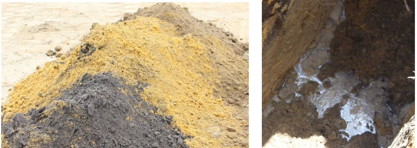
Figure 4.2 (L) Excavated soil showing layers. (R) Water seepage at 2.2 m.
