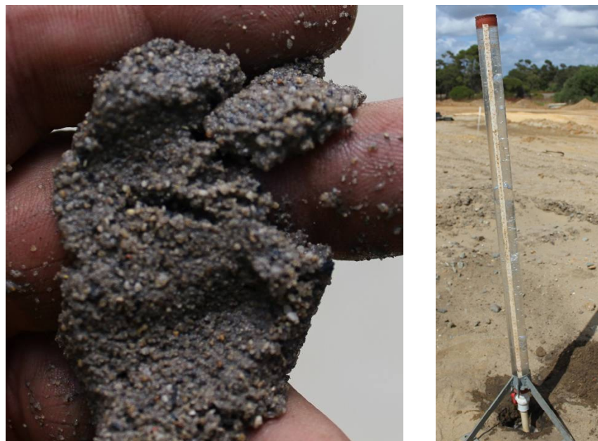
Figure 4.4 (L) Ribbon test TP1. (R) Permeability determination (very rapid bubbles).
