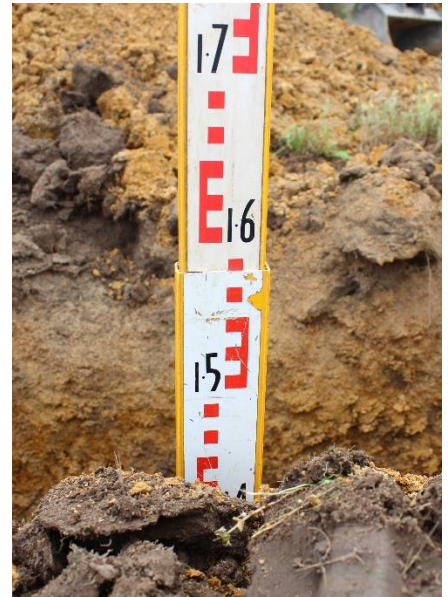
Figure 4.8 (L) Soil profile for test pit 2. (R) Depth to 1500 mm, hard digging.
