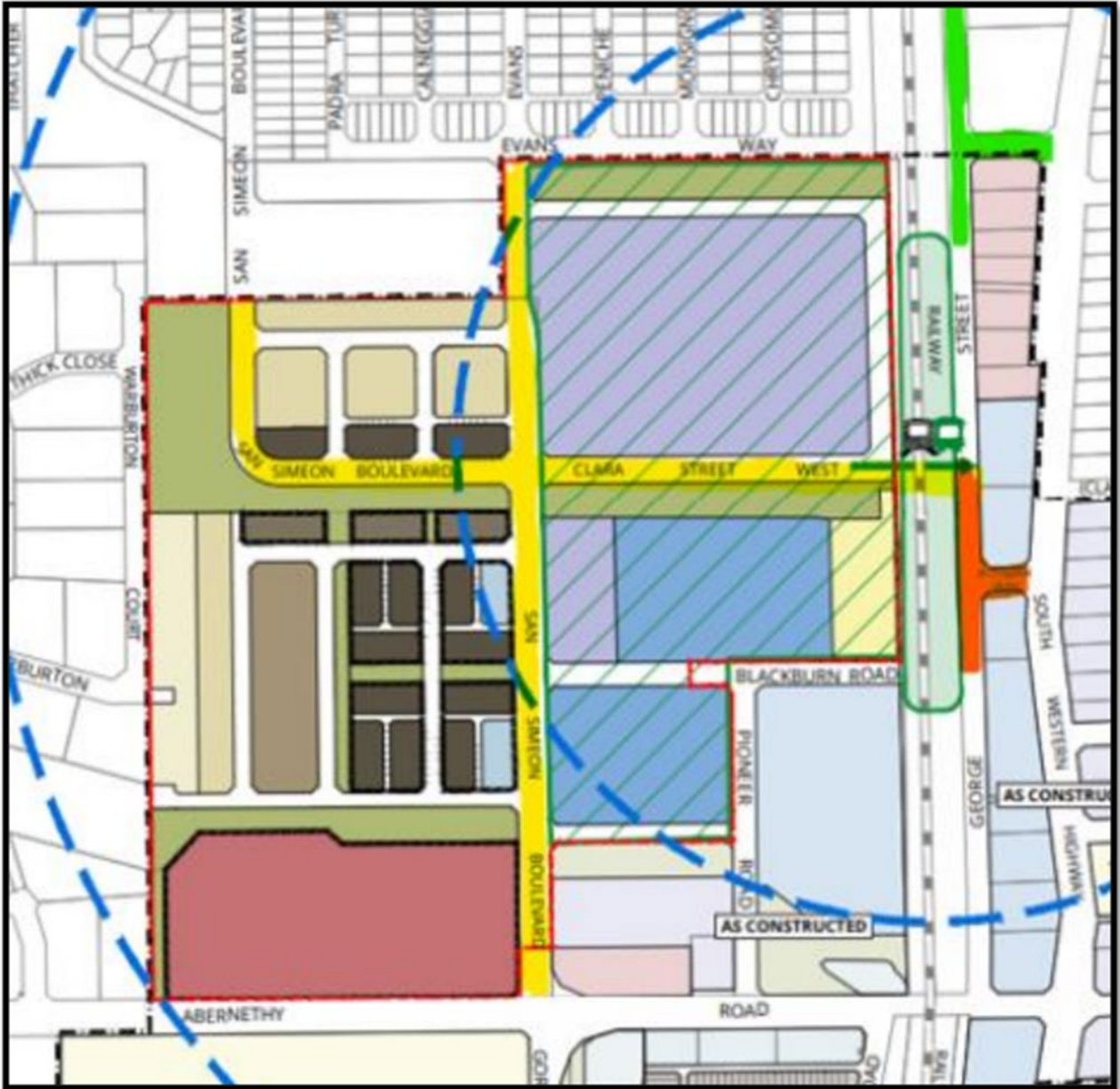
Highlighted areas form road infrastructure being delivered
