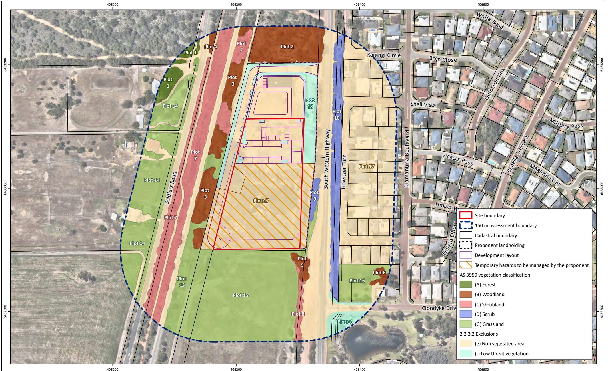
Figure 3: Post Development Site Conditions - AS 3959 Vegetation Classification Project: Bushfire Management Plan Portion Lot 128 South Western Highway, Byford Client: Parsons Management Group Pty Ltd
