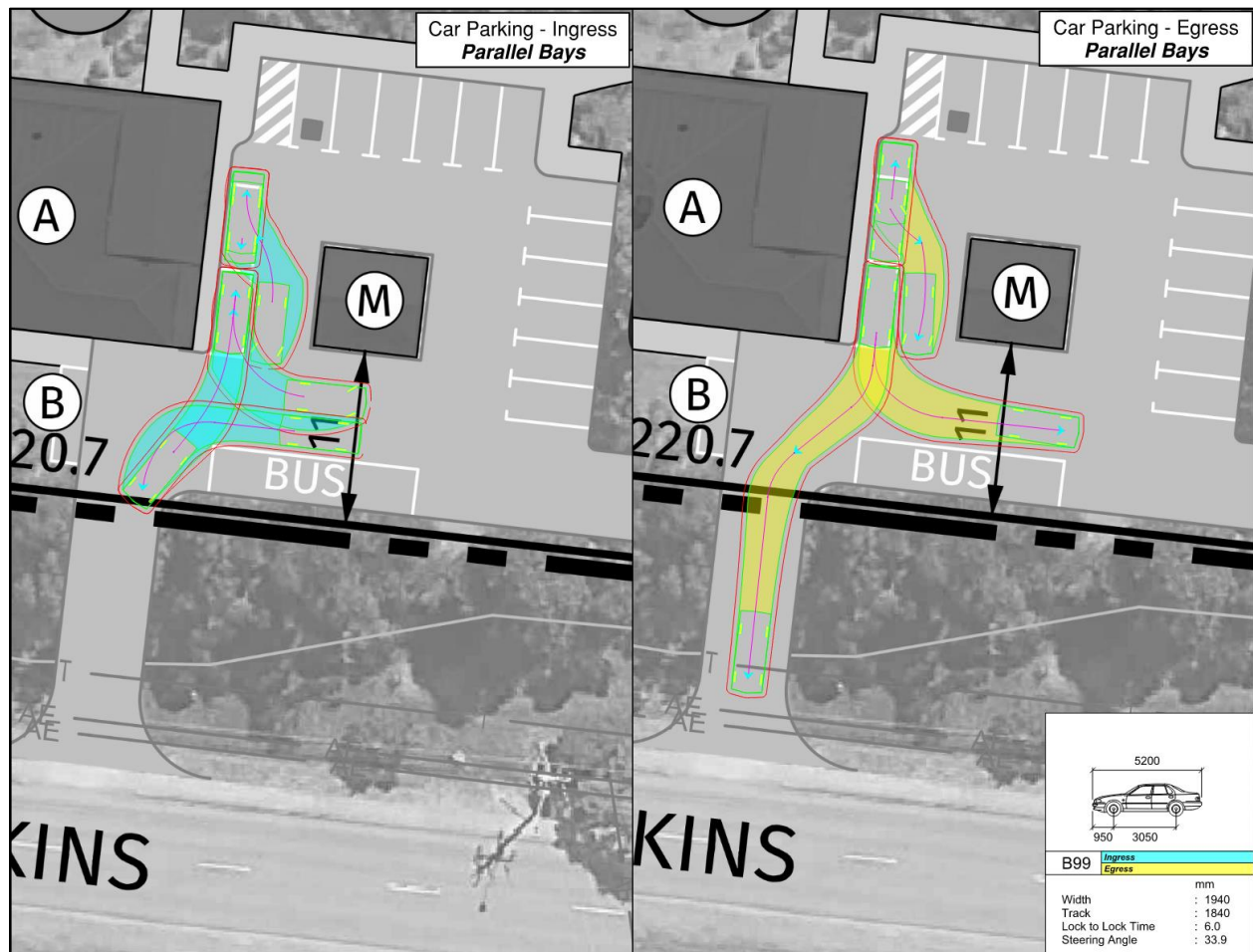
Figure 4-3 Swept Path - Parallel Car Parking Bays
