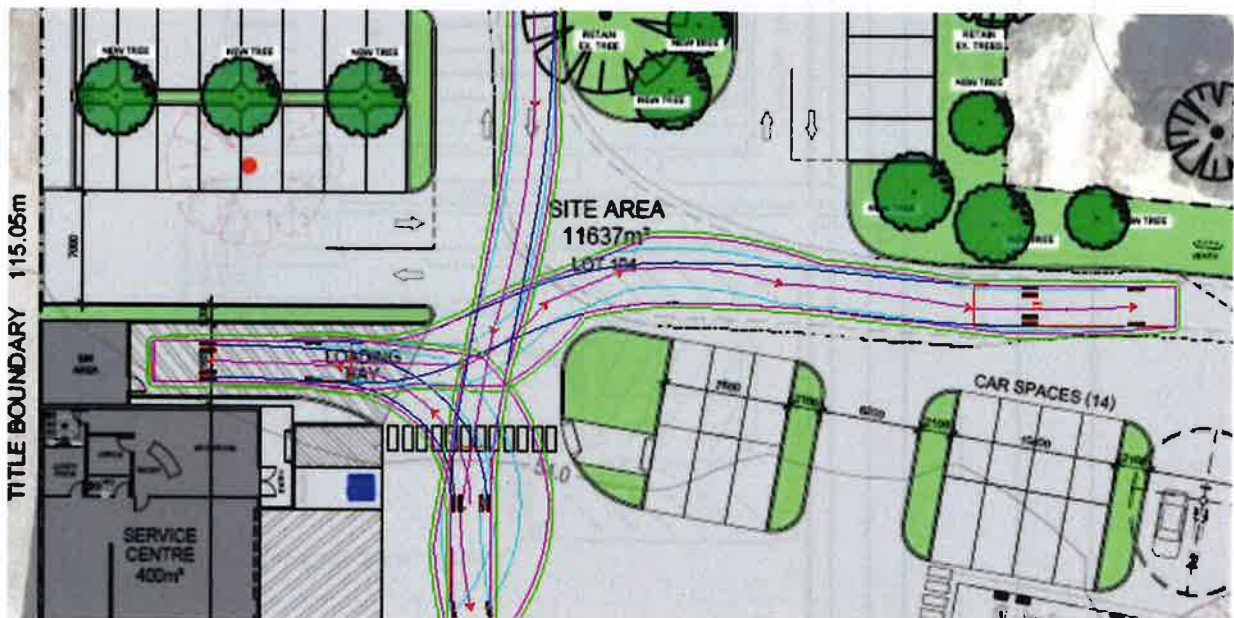
Figure 46 - Assessed swept path of 12.5 m HRV reversing into Restricted Retail Loading Bay and driving forward out onto George St (in colour – black outline is swept path of 19 m ST Fuel Tanker)
