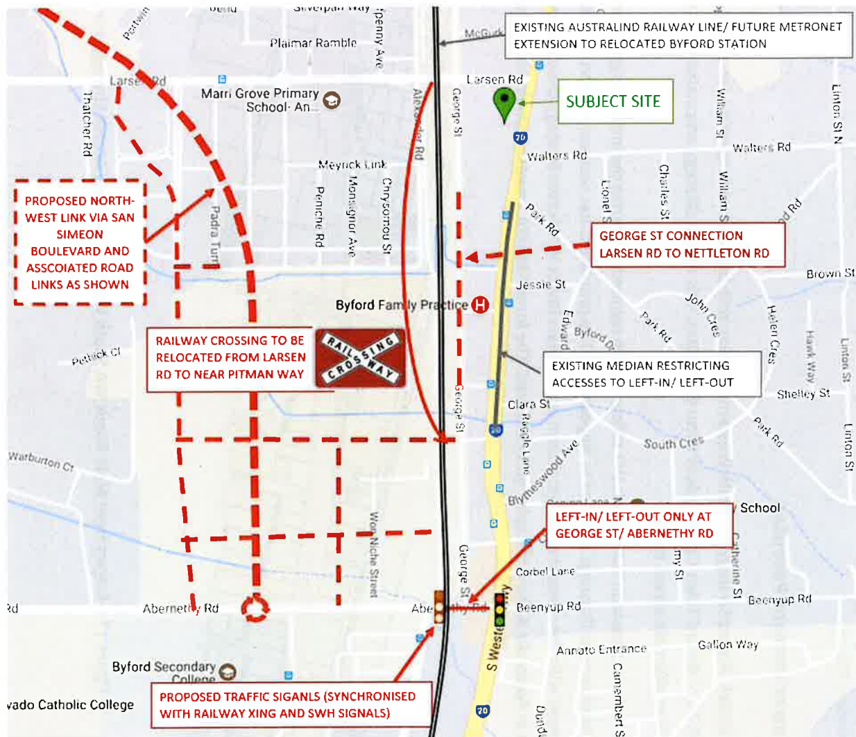
Figure 16 – Summary of road and public transport network proposals in vicinity of the subject site
