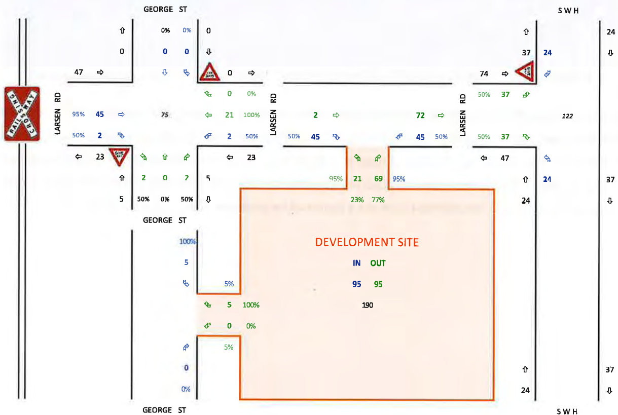
Figure 25 – Forecast 1 PM – 2 PM midweek Trip Generation, Distribution and Assignment
