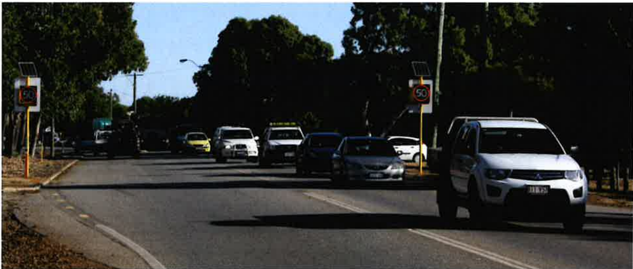
Photograph 3 – Looking south on South Western Hwy to 50 km/h variable speed limit signs before Larsen Rd
