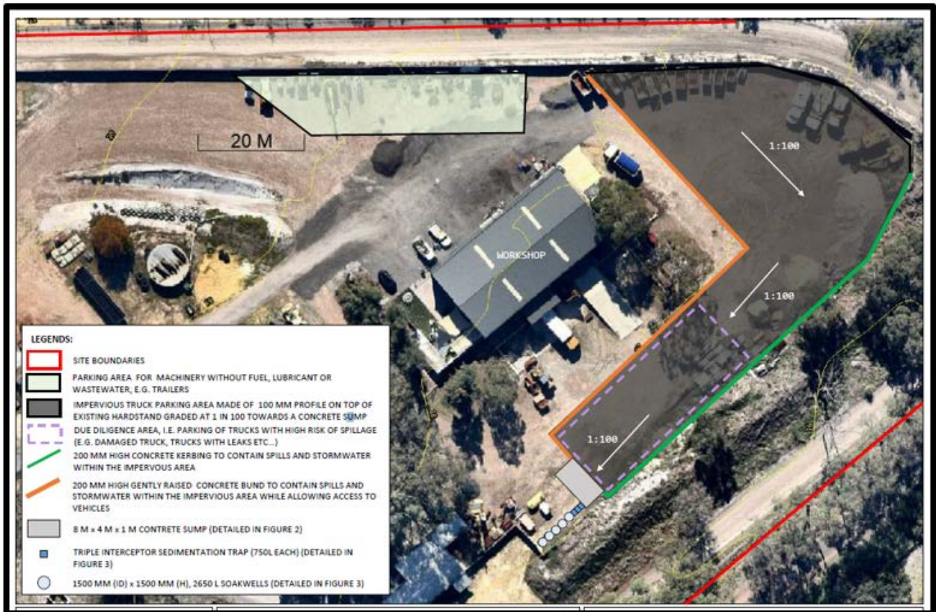
Figure 4: Proposed spill and Stormwater Management System
