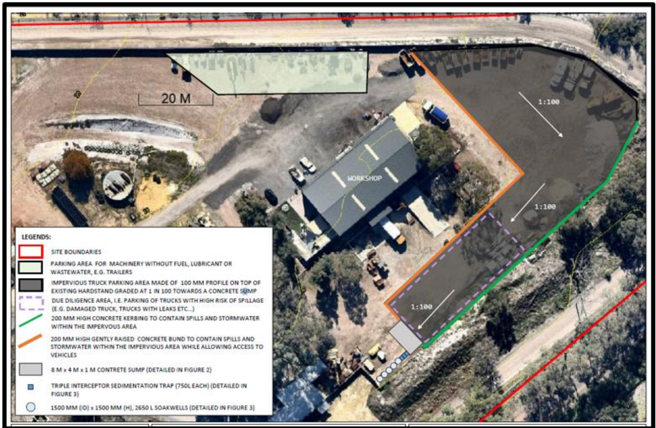
Figure 4: Proposed spill and Stormwater Management System
