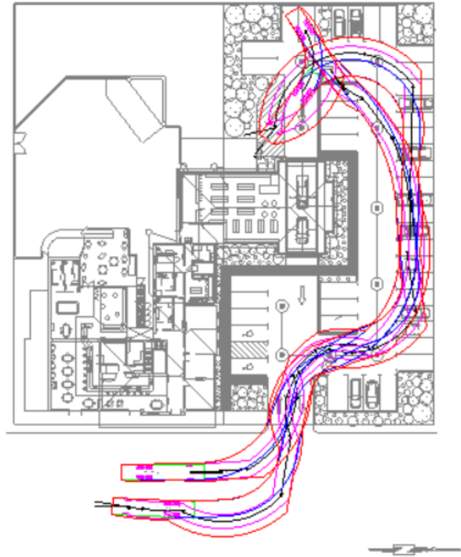
Figure 9: Turn path of a 12.5 m service vehicle undertaking a front-in, front out manoeuvre.
