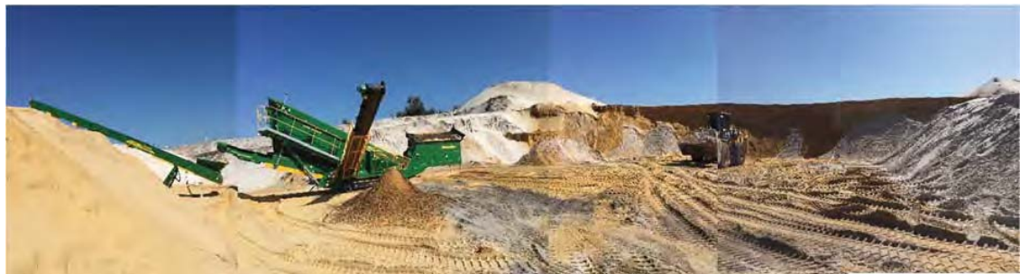
FIGURE 2 – LOADING AND SCREENING OPERATIONS WITHIN A PIT (SIMILAR SAND EXTRACTION TO PROPOSED OPERATIONS)
