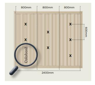
Annotation of fencing panelling above. Please note – application is for two (2) of the above sections – equalling a total of 4.8m metres.
