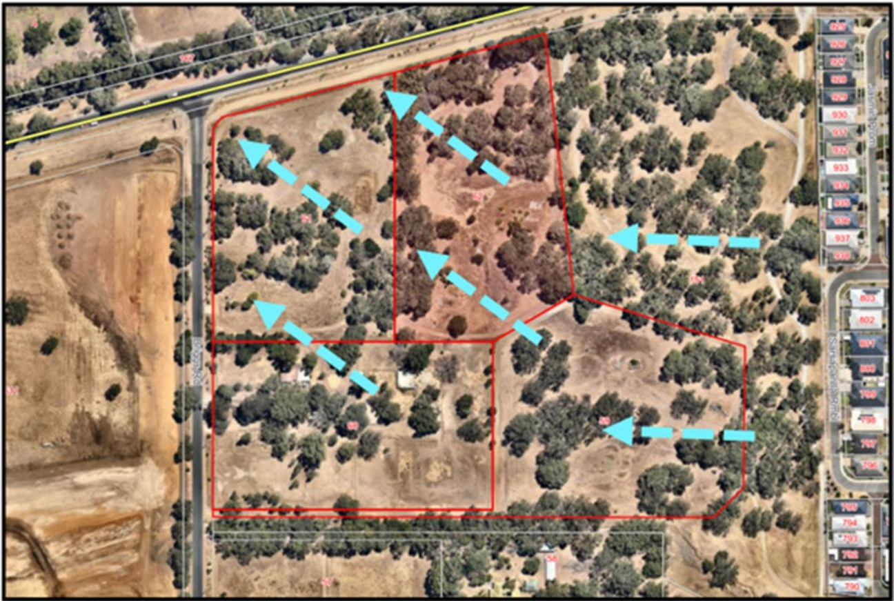
Figure 10: Existing natural surface/groundwater movement (blue) towards the North-West corner of the lot
