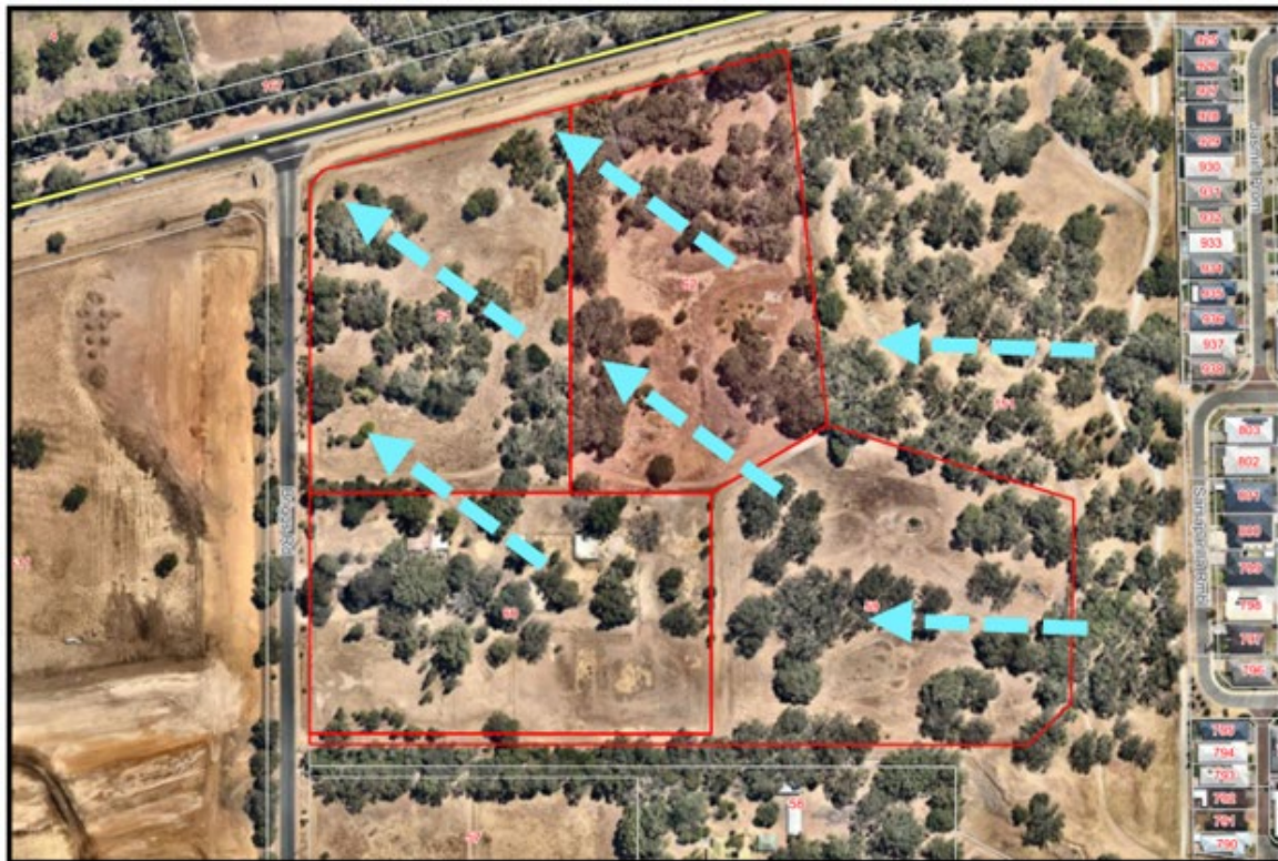
Existing natural surface/groundwater movement (blue) towards the North-West corner of the lot
