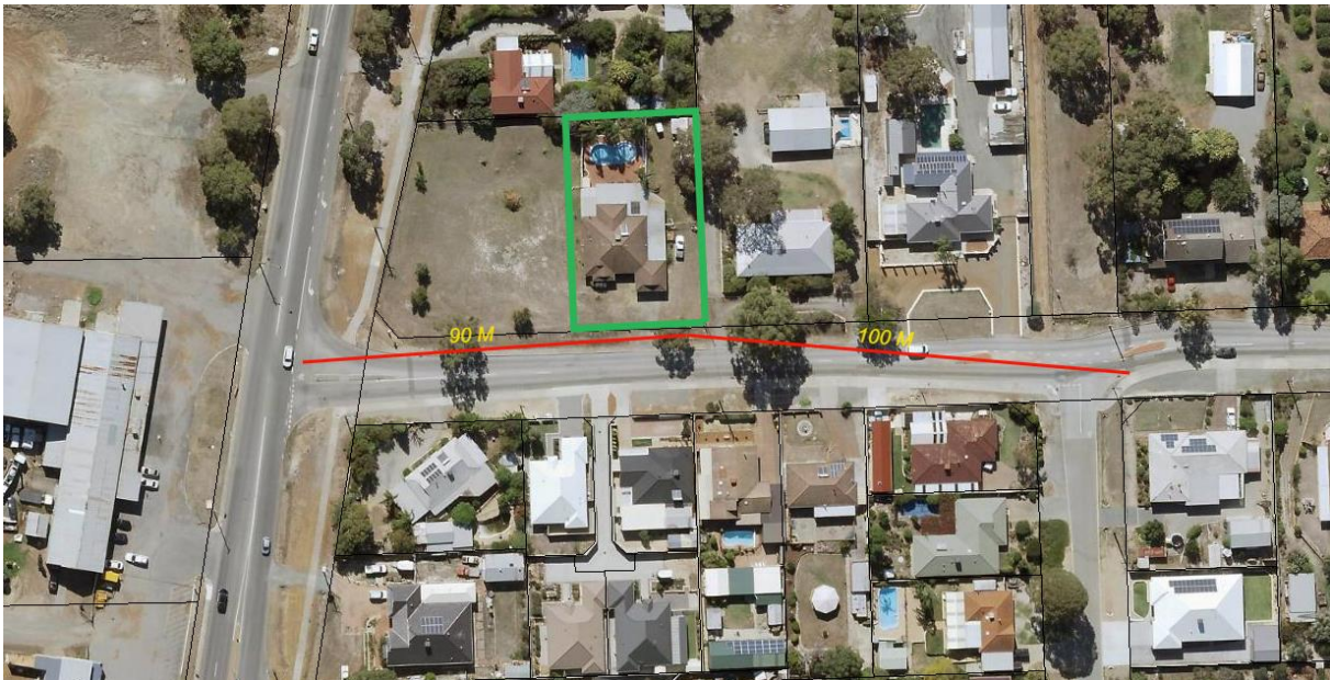
Figure 10: AS2890.1 – Access Sight Distance
