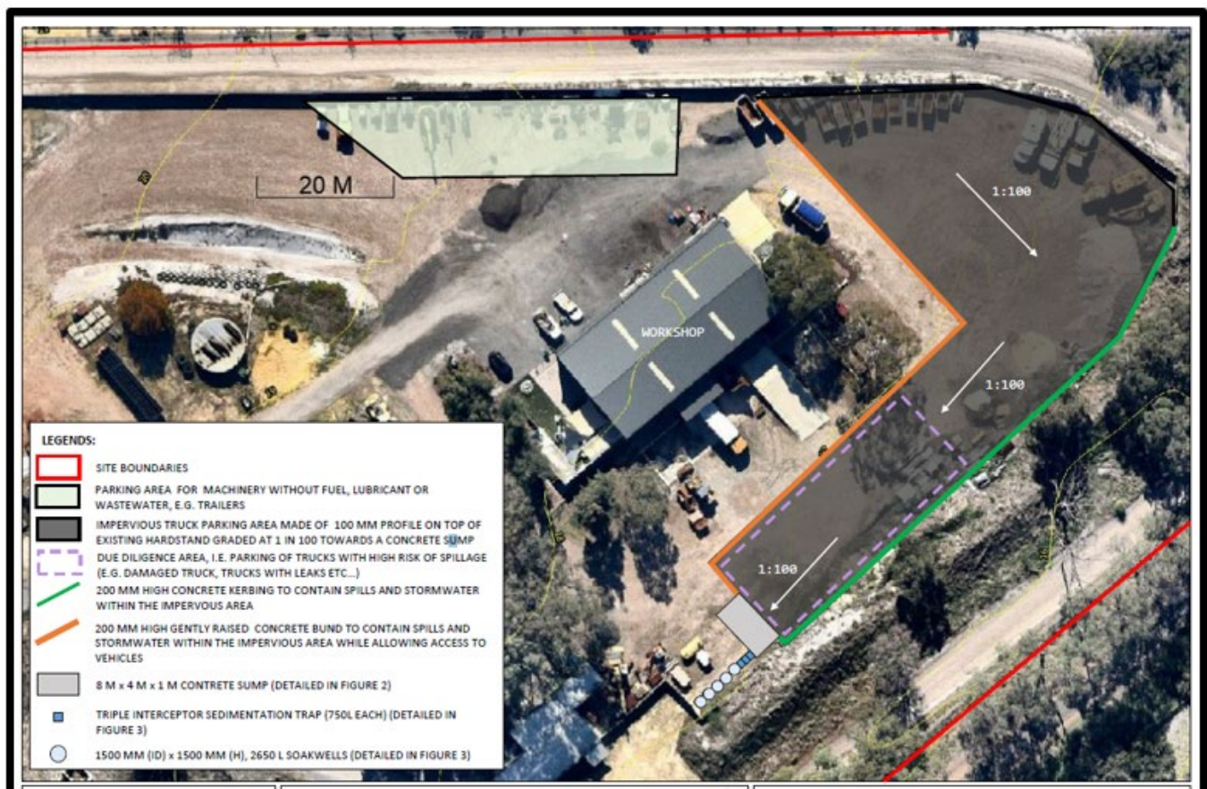
Figure 4: Proposed spill and Stormwater Management System
