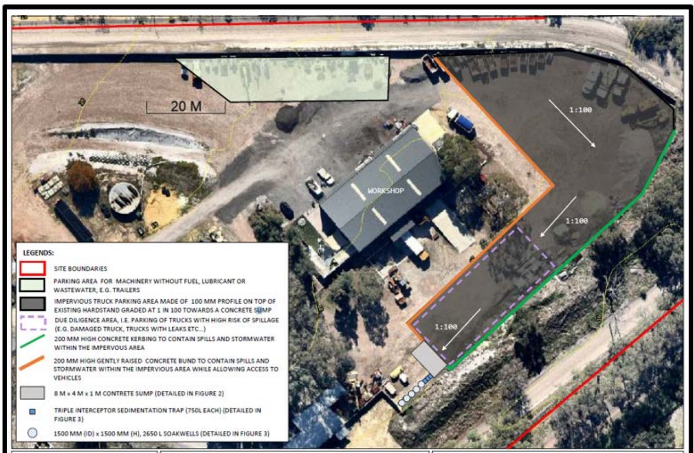
Figure 4: Proposed spill and Stormwater Management System
