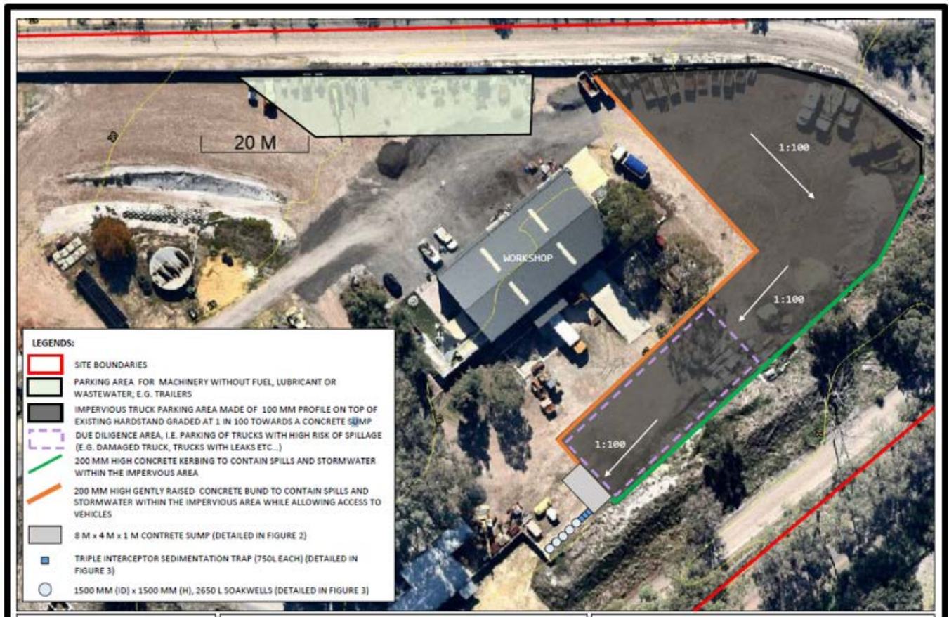
Figure 4: Proposed spill and Stormwater Management System
