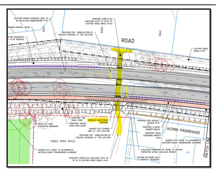
This trail (upon completion) would be able to be a granular type pavement, and also provide equine riders an environment for riding which is further removed from the (future) extension of Sansimeon Boulevard, and the rail corridor.
