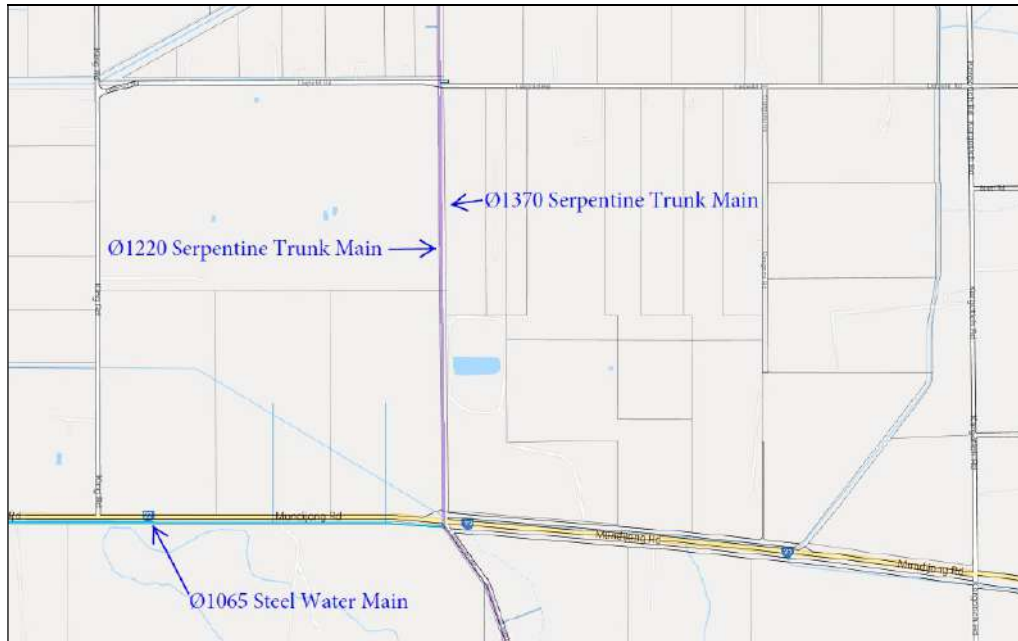
Figure 2 – Primary Water Infrastructure
