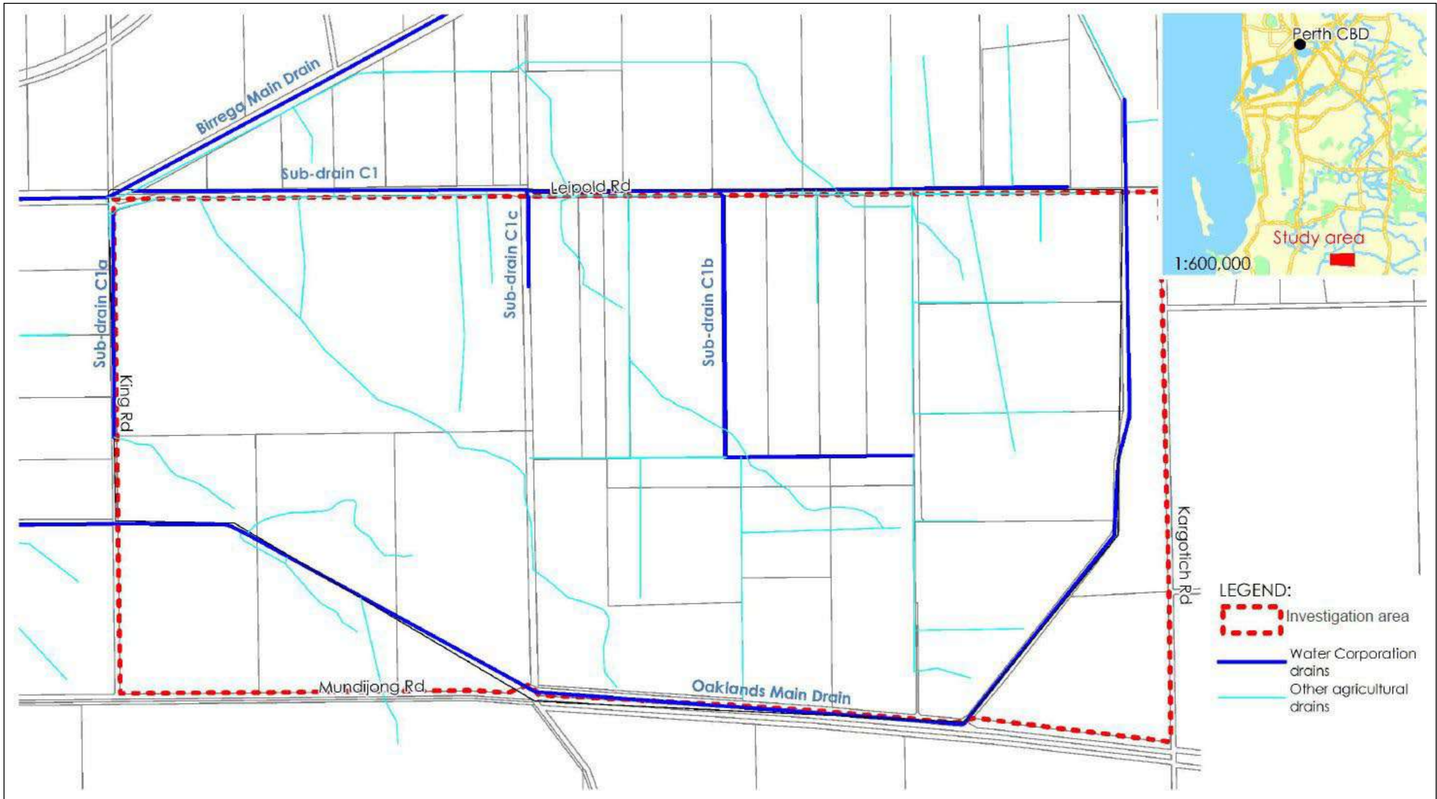
Figure 9 Major and Minor Drainage Lines
