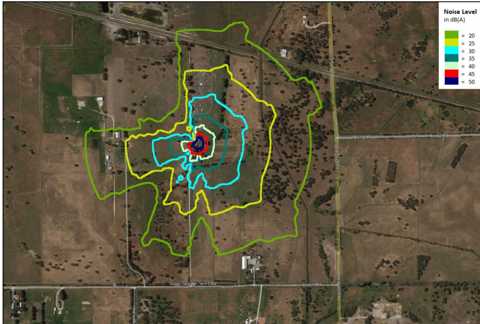
**Figure 7: Worst-case day-time noise level  $L_{A_{Max}}$  contours for scenario 4.**
