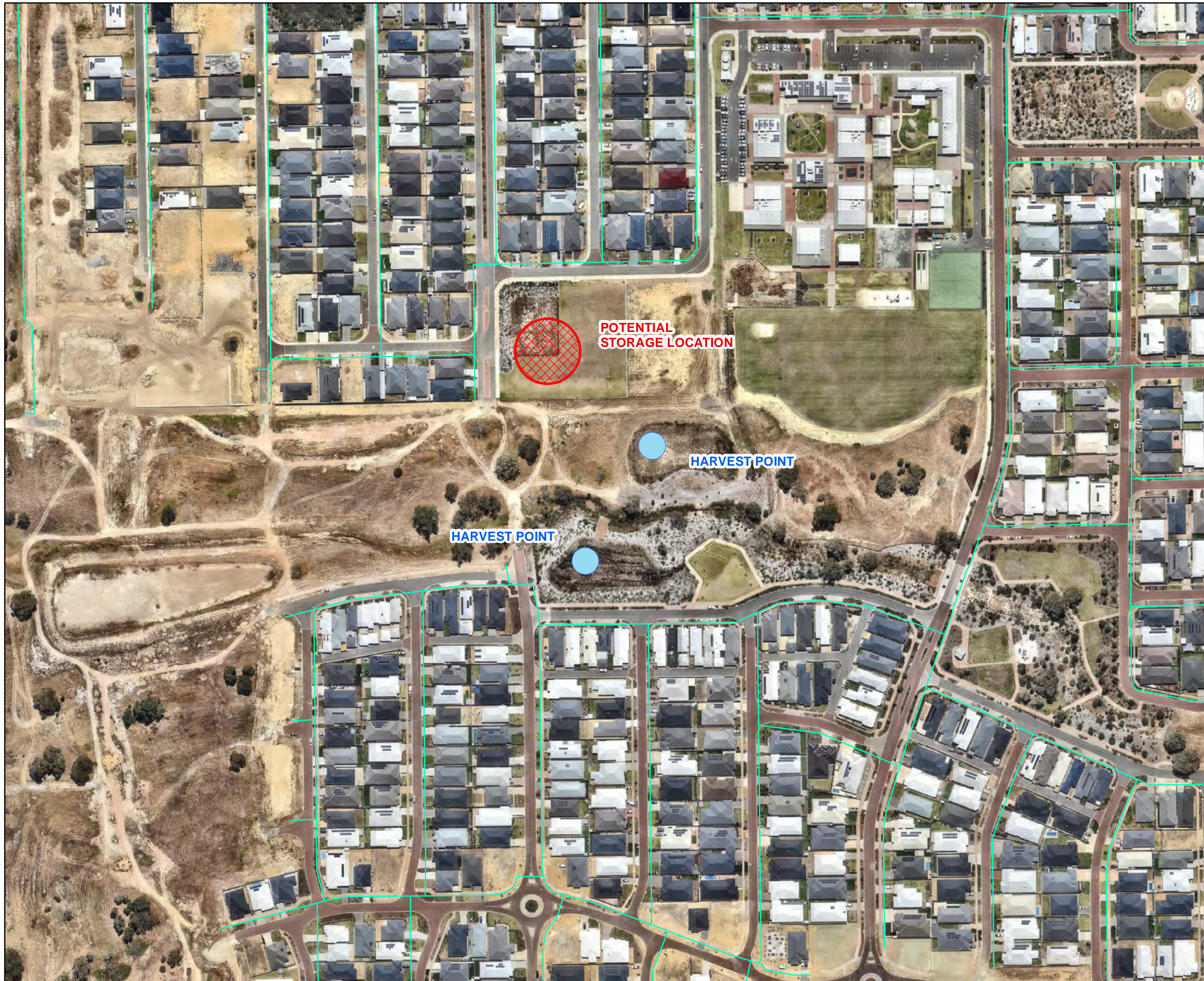
Figure 12 Option 3- Surface Water Harvesting at Woodland Grove Sporting Facility
