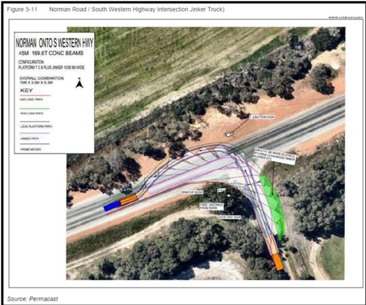
45m Jinker truck swept path diagram - left turn from Norman Road onto South Western Highway
